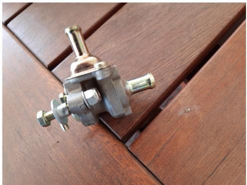
• Now make a blanking plate to cover the inlet into the exhaust. Thick aluminium is sufficient, use the fitting that came off as a template. I made a gasket using gasket paper and gasket goo to seal it. The existing bolts are a bit long so you can either use washers under the head of the bolts or use shorter bolts or assault them with your trusty Dremel. I used three washers.
